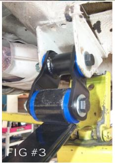
ONCE THE CROSSMEMBER IS INSTALLED, ALL HARDWARE MUST BE TIGHTENED TAKING INTO CONSIDERATION NOT TO OVER-TIGHTEN THE UPPER BELL SHACKLE BOLTS AS THEY CAN BIND.
