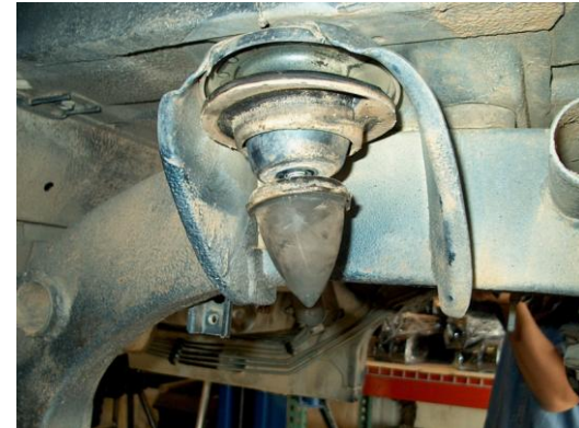
Remove all four factory bump stops & rubber coil spring bushings.
