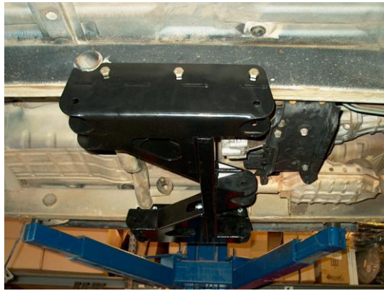
24. Bolt in place using six 1/2 -20x3 1/4" bolts & nylocs. Center crossmember between subframes and tighten the four 1/2 -20x1x1/4" bolts.
