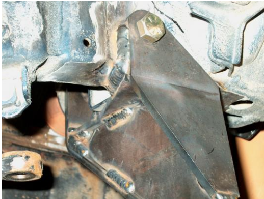
26. Weld bracket to frame as shown.
