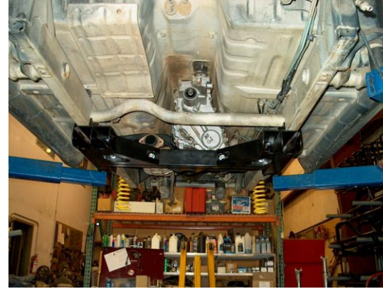
24. Bolt in place using six 1/2 -20x3 1/4" bolts & nylocs. Center crossmember between subframes and tighten the four 1/2 -20x1x1/4" bolts.
