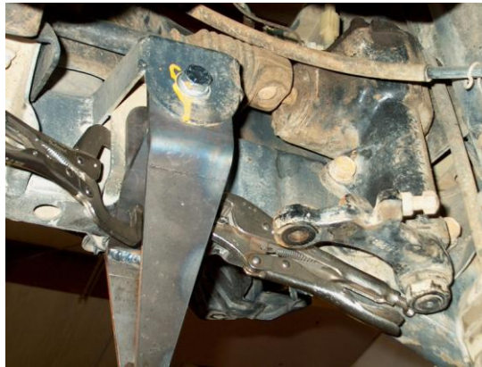
25. Fit panhard bracket up to drivers side frame rail. The bracket fits snugly into pocket where the front differential housing bracket used to be (just back from the steering box). Make sure the bracket seats up against the bottom of the frame. Clamp if necessary. Install one 12m-1.25 bolt through the factory frame hole. Drill one 1/2" hole through the frame rail using the panhard bracket as a drill guide. Unbolt and clean paint and undercoating from the frame in the area around the bracket. Bolt the bracket back into place using supplied 12m – 1.25x90 bolt, lockwasher and one 1/2 -20x3 1/4" bolt, flatwasher and nyloc.
