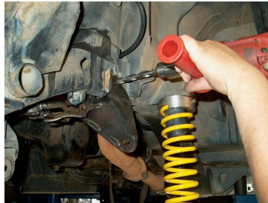
25. Fit panhard bracket up to drivers side frame rail. The bracket fits snugly into pocket where the front differential housing bracket used to be (just back from the steering box). Make sure the bracket seats up against the bottom of the frame. Clamp if necessary. Install one 12m-1.25 bolt through the factory frame hole. Drill one 1/2" hole through the frame rail using the panhard bracket as a drill guide. Unbolt and clean paint and undercoating from the frame in the area around the bracket. Bolt the bracket back into place using supplied 12m – 1.25x90 bolt, lockwasher and one 1/2 -20x3 1/4" bolt, flatwasher and nyloc.
